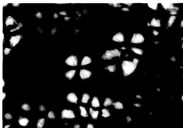
Figure 9 Positive non-ringed spherulites grown at 185°C in the 60/40 composition after fusion at 280°C for 5 min
